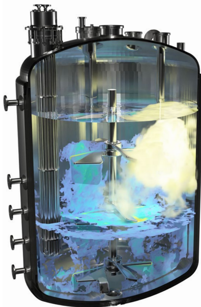
① CFD simulation of a BE6300 with a 3-stage TAR/TAF agitator system. Visualisation of the flow velocity and injection of a second substance (yellow).
