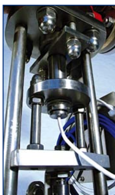
Temperature probe, flexsens 100, can be removed laterally without having to dismantle or open the valve
