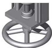
Standard: Inline actuator unit with stainless steel cover
